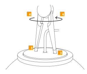
5 Once cap is loose, use fingers to unscrew and remove the cap. Gently slide the cap and stem away from fixture.
